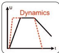
For applications where a fast variation of voltage from a high to a low value is required, models from 1kW and up to 360V output voltage can be equipped with a two-quadrants power-sink module (active load). This improved dynamics is achieved by the capability of this power-sink module to faster discharge the internal capacitors as well as the filter capacitors of the connected equipment.
