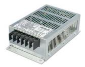
This rugged, industrial quality AC/DC power supply uses field-proven technology to generate the required output power. It is a mature product with a track record in numerous applications. The input accepts any AC voltage from 95V to 264Vac. Cooling is via baseplate to a heat-sinking surface and by natural convection. Low component count, large design headroom, and the use of components with established reliability result in a high MTBF.
