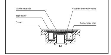
During ordinary use of the battery, the vent valve is closed to shut out outside air and prevent oxygen in the air from reacting with the active material in the negative electrodes.
