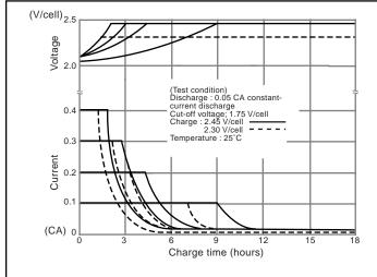
In order to fully utilize the characteristics of VRLA batteries, constant-voltage charging is recommended. For details of charging see page 20.
