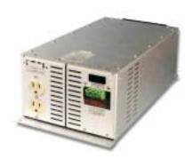
The SFC1000 Series is a highly compact AC/AC frequency converter. Suitable for a wide range of applications, the SFC1000 features full electronic protection, high efficiency and low output noise. Well established design techniques are used to ensure high reliability. The 1000VA converter is cooled by a built-in fan. Extended operating temperature (-40 to  $\pm$ 65°C) is available.
