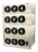
The STT 12000 AC/AC frequency converter provides 3-phase power from a 3-phase line outlet. The standard unit delivers 3-phase outputs of 208rms, 380Vrms or 415Vrms (PH-PH) continuous at 50, 60, or 400Hz. The floating outputs are isolated from each other and can be connected in a 'Y' configuration or left as three individual outputs. In 'Y' configuration, the centre point (neutral) can be grounded. The unit features full electronic protection, high efficiency and low input and output noise.
