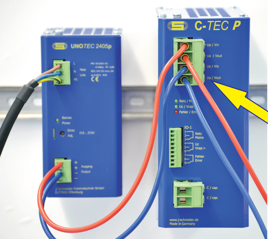
Connect the load to the buffered 24 V DC output of the C-TEC
