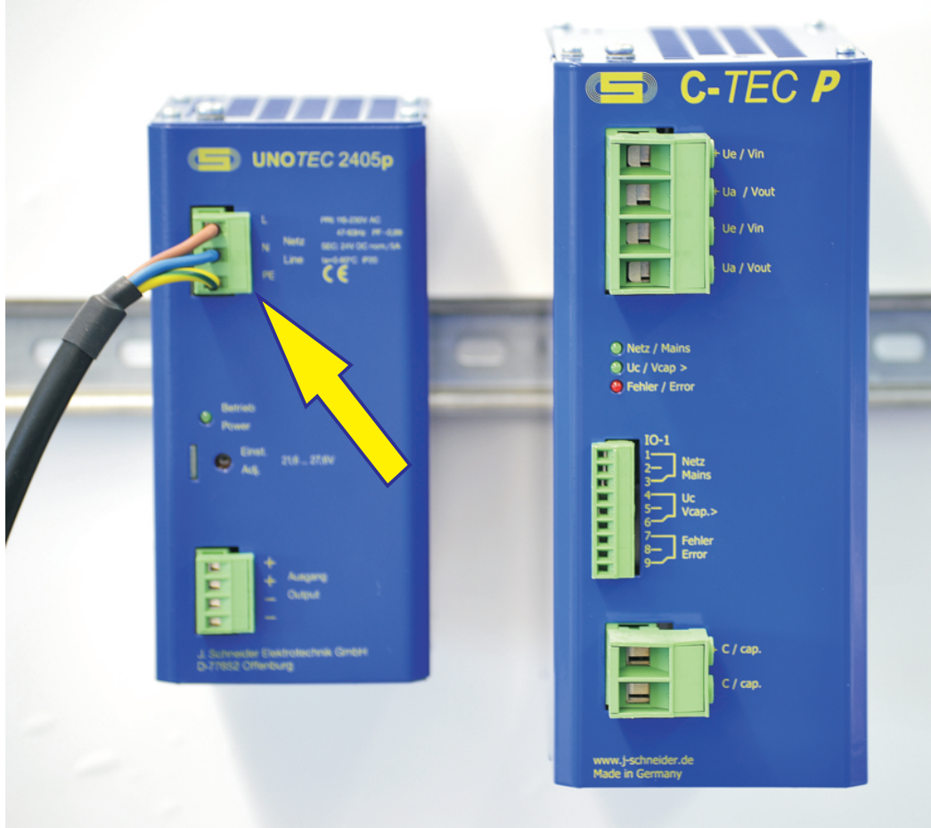
Connect the 24 V DC power supply to the mains (230 V AC)
